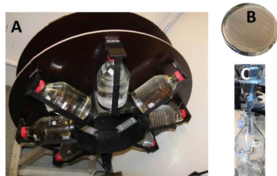
Fig. 1. A slowly rotating carousel system with two units containing eight 2-L flasks with test solutions and with 300 mL headspace in the flasks (A). In experiments with marine particles, samples (100 mL) were filtered through steel filters with mesh size 20 \mu\text{m} (B) to separate particles/aggregates and filtrates (C).
